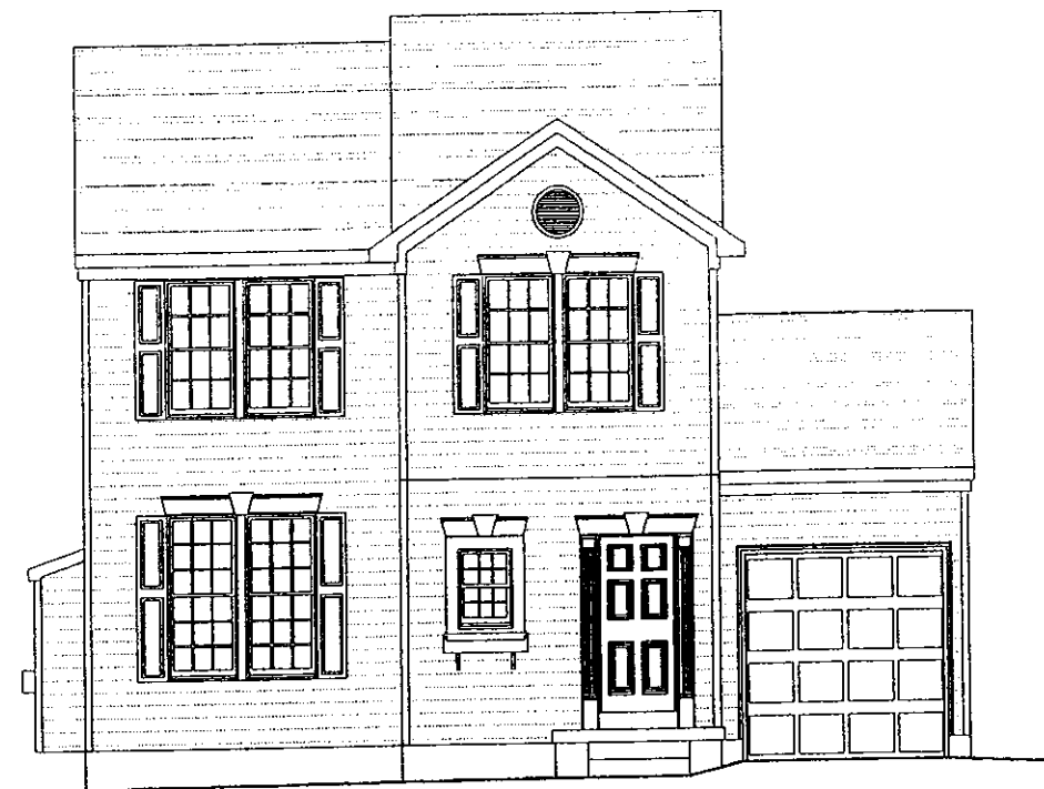
Elevation "A" (shown w/opt. garage, fireplace, & 2' cantilever)
